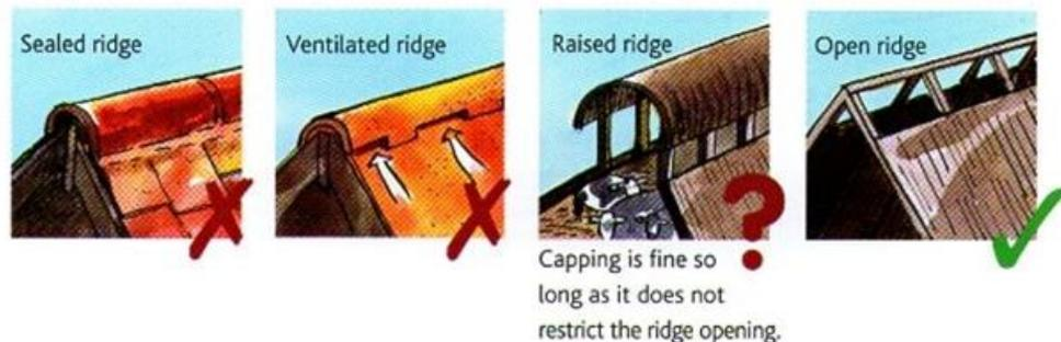
One of the best ways to improve any livestock building is to remove the ridge, leaving open space. This will improve ventilation markedly and lead to improved animal performance. The 'chimney' effect prevents significant rain entering the house. Even over a wet winter housing period the amount of extra moisture entering through an open ridge will be small compared with that produced by housed stock - less than 5%.
